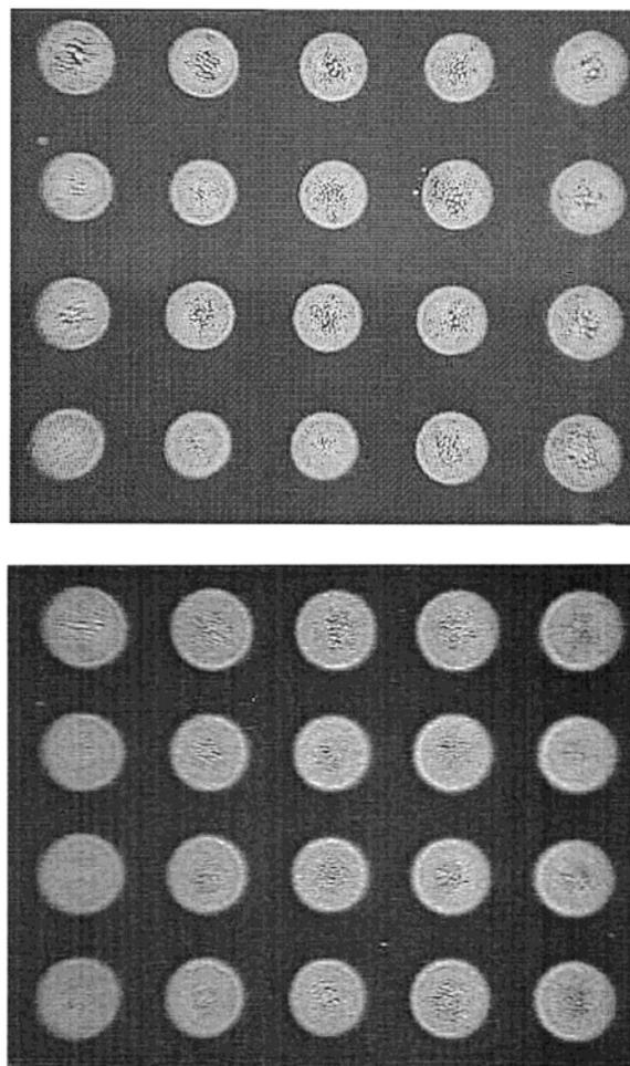
Figure 4. LDH spots that are sprayed 400 μm apart (center to center) using a distance between the capillary tip and substrate of 300 μm; (A) flow rate, 140 pL s<sup>-1</sup>; (B) flow rate, 280 pL s<sup>-1</sup>.
