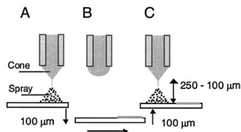
Figure 2. (A) Schematic view of the cone-jet mode. (B) Spraying stops due to an increase of the distance between the tip and substrate. (C) Spraying resumes.
