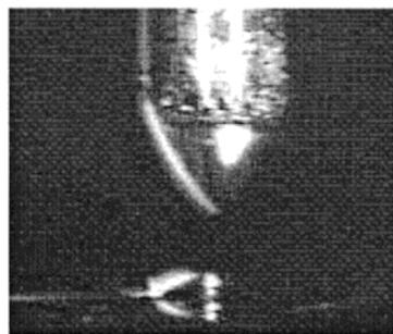
Figure 3. ESD of a small spot 130  $\mu\text{m}$  in diameter. The distance between the capillary tip and the substrate is  $\sim 220 \mu\text{m}$ . The cone-length is 130  $\mu\text{m}$ .
