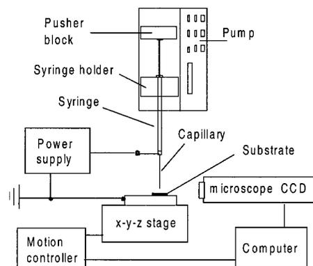
Figure 1. Schematic diagram of the ESD system.
